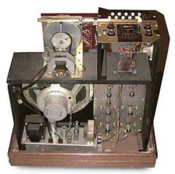
fig. 101 The Wurlitzer Sideman (open casing showing internal speaker, rotating disk and circuitry)
