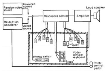
Fig. 53 Diagram of the "Voder"
