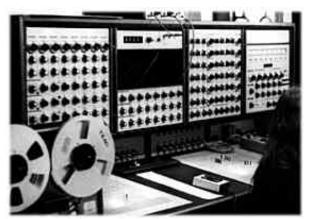
fig. 137 The EMS Synthi 100.12 VCOs, 2 keyboards and a 256 step sequencer
