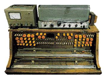
fig. 38 Dr. Friedrich Trautwein's "Trautonium" showing the fingerboard wires and the metal rails.
