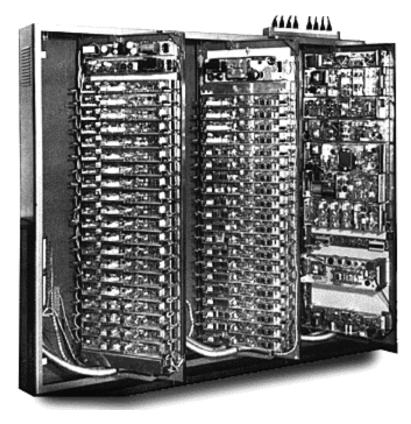
fig. 95 A Siemens Vocoder opened to show circuits
