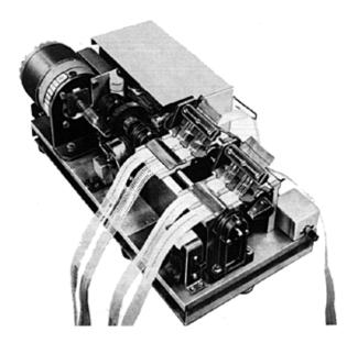
fig. 94 The Siemens punch-tape control mechanism
