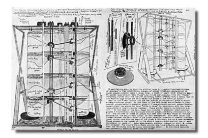
fig. 72 The Kangaroo Poutch Free Music Machine (Grainger's diagram)
