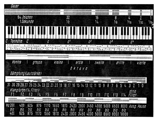
fig. 97 "Fig.1" shows the coding scheme of the paper roll controller: 4 parallel-run strips (similar to the way they are used with a telex machine ) containing the musical information for a voice or level in binary code.
