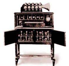
fig. 26 The Pianorad, showing oscillators and speaker horn
