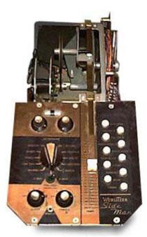
fig. 102 The top panel of the Sideman showing (L-R) pattern select control, tempo slider and manual triggers
