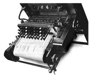
fig. 82 The punch-paper keyboard input of the RCA MKII
