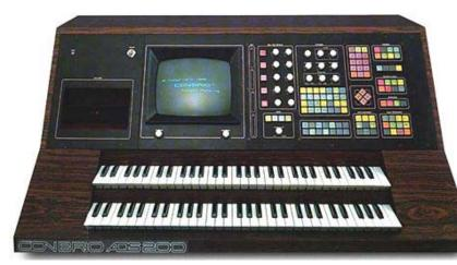
In 1982 Con Brio released the ADS 200-R a 32 voice (expandable to 64) featuring a 16-track polyphonic sequencer with 80,000 note storage capability with 'editing functions' available from the scoring screen.
