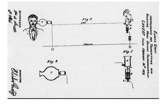
fig. 3 Gray's drawing for the patent of a method for "transmitting vocal sounds telegraphically"
