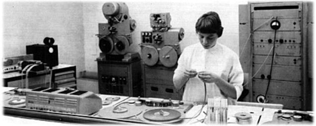
fig. 96 The machine room at the 'Studio for Electronic Music' (L-R:punch-paper controller, 2 four channel magnetic tape recorders, 'Bildabtaster' picture-scanner. Foreground:2 Master magnetic tape machines)
