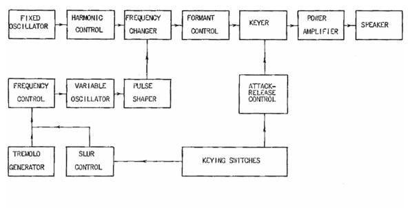
FIGURE 1 - BLOCK DIAGRAY OF ONE WOLCE CHANNEL fig. 75 "Figure 1"
