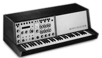
fig. 135 EMS Synthi Sequencer 256. 256 Event x 42 bit Memory sequencer (1971)
