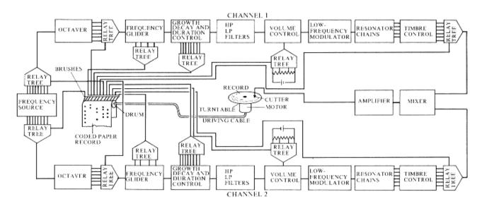
fig. 83 A diagram of the RCA MkII showing hard disk recording and paper roll programmer.
