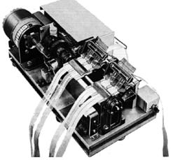
fig. 99 The punch-paper strip controller
