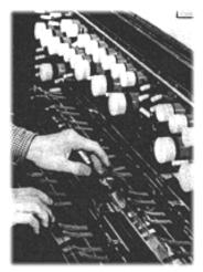
fig. 39 The Mixturtrautonium showing the resistance wires with leather thongs.
